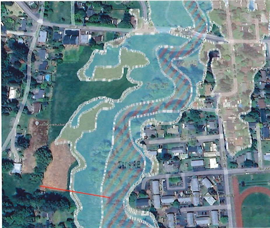
Figure 1. FEMA-identified flood areas for the proposed Buxton Ranch development. The red line represents the approximate southern boundary of the development. Red-hatched areas represent the creek and floodway. Light green areas represent the 100-year floodplain. Tan areas represent the 500-year floodplain and approximately 129,000 square feet.
