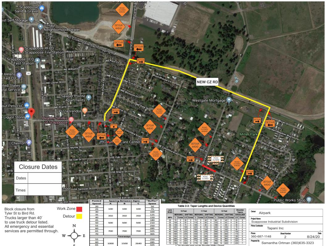
"L" for shoulder taper equals Shoulder Width x Speed Figures shown are for 10' shoulders.
