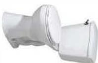
Check your toilets for leaks. Drop a dye tablet or a teaspoon of food coloring in the tank. If the color appears in the bowl after 15 minutes, replace the "flapper" valve.
