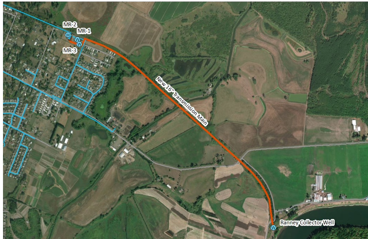
Figure 4.4 Ranney Collector Well Location and Transmission
