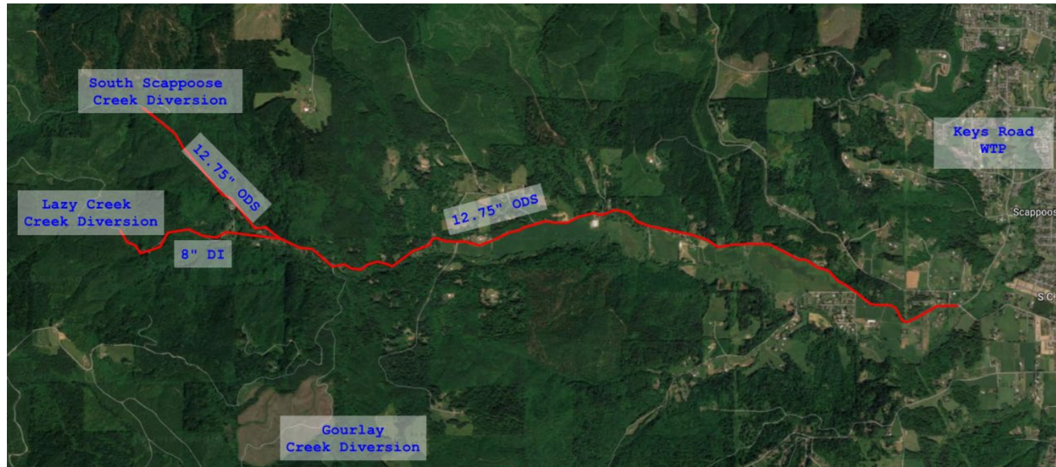
Figure 4.1 Transmission Main Replacements for Maintaining Surface Water
