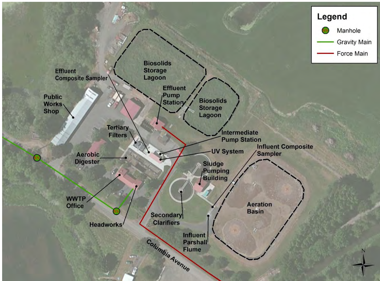
Figure ES7 – Existing WWTP Layout
