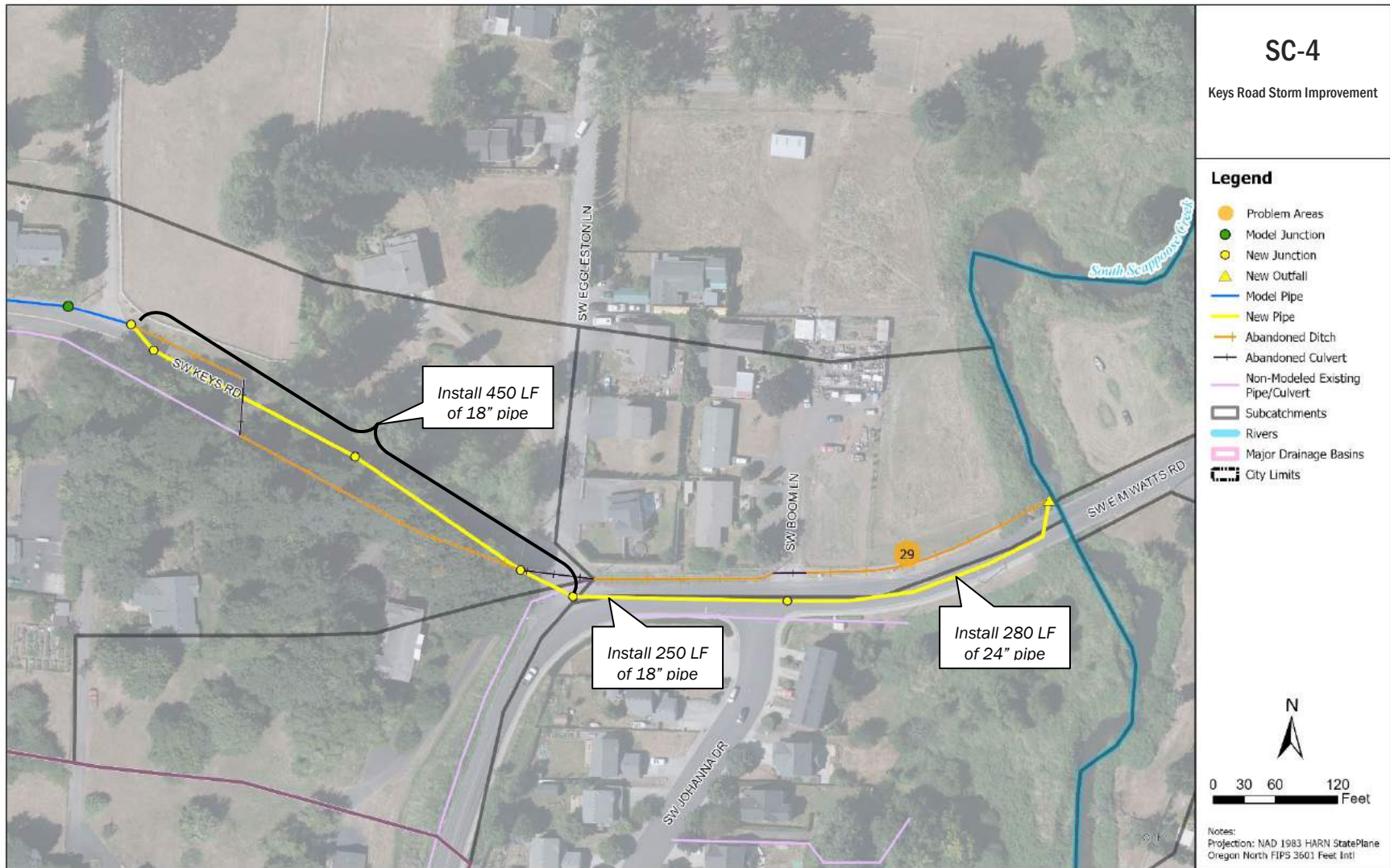
Figure 6. SC-4: Keys Road Storm Improvements
